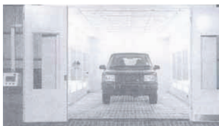
Figure 4 Typical spray booth for vehicles
